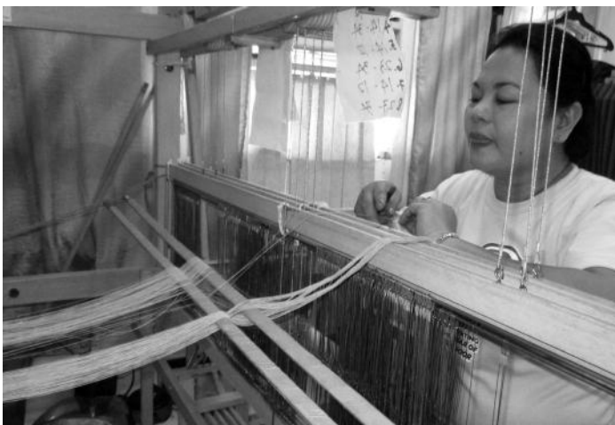
Celia doing the third step in hand-weaving, drawing-in
